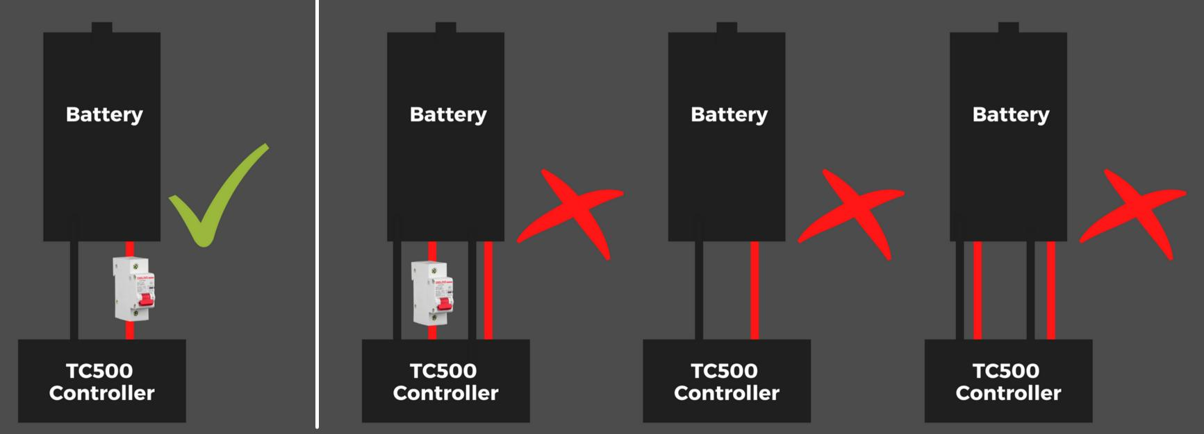
You should NEVER use the Controller without the stock fuse! It is dangerous and can cause serious damage!
